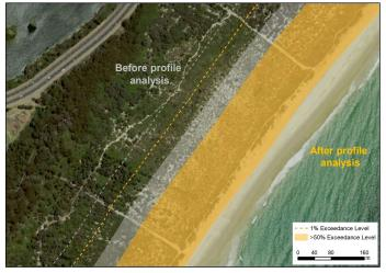
Example of a reduction in future shoreline change predictions where the potential Bruun effect was found to be lower after profile analysis using high-resolution seabed mapping
